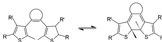
Figure 1. Schematic representation of photocyclization/cycloreversion in a diarylethene based on thiophene aryl groups. The central double bond is included in a cyclic structure (usually penta-atomic, schematized by the circular fragment) that prevents cis–trans photoisomerization.
